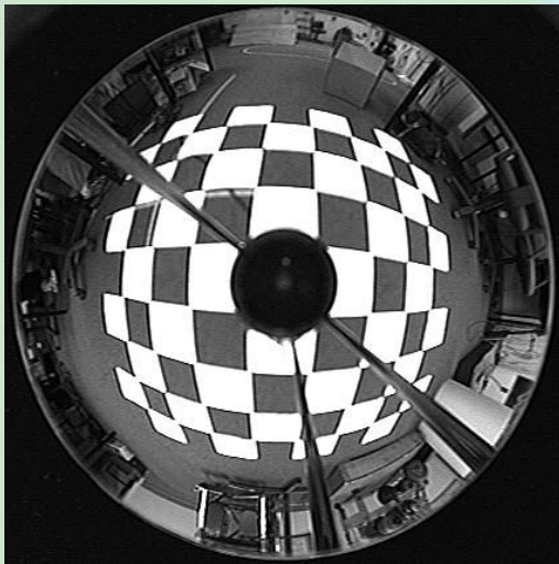
Warped view of the environment obtained with a parabolic mirror.
