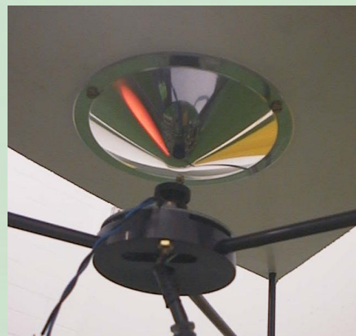
A video camera looking into an omnidirectional mirror.
