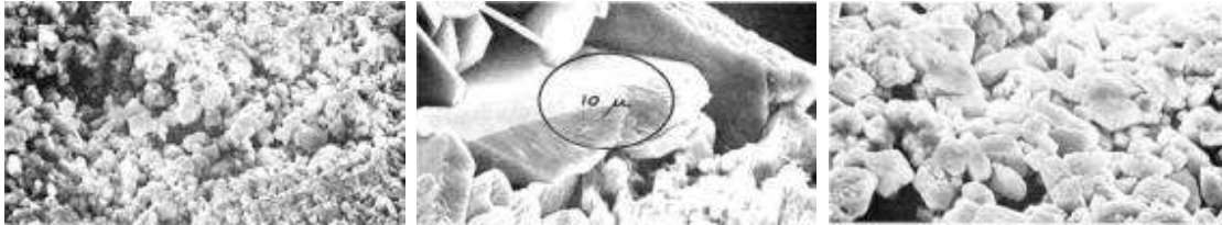
Electron photograph of a NiCd electrode. To the left, original state of the electrode with many cadmium hydroxide crystals. In the center a large crystal has developed and the capacity of the battery has fallen by around 20%. To the right, the state of the reconditioned battery.
