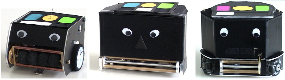
Fig. 1. Different robots designs. From left to right: classical two wheeled design, two wheeled defender, and robot with omnidirectional drive.
