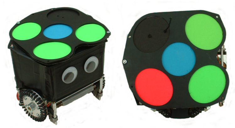
Figure 3.3: The color markers of the small size robot as in 2004. In the middle is the mandatory team marker (blue or yellow), the other markers code the orientation of the robot and its identity number.
