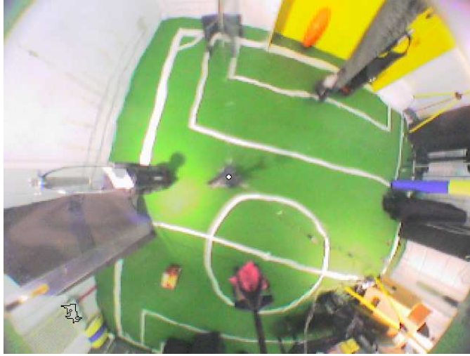
Figure 3.6: In this bright image the same color values are found on the field, in the ball, and in the yellow goal. Therefore the same color value can be assigned to multiple color classes.
