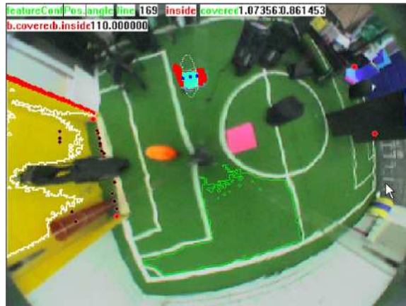
Figure 3.5: Grown regions which fail to meet the validation criteria. Pixels of the goal-box and ball regions are outside the expected region, or the field region does not cover a required percentage of the expected region.
