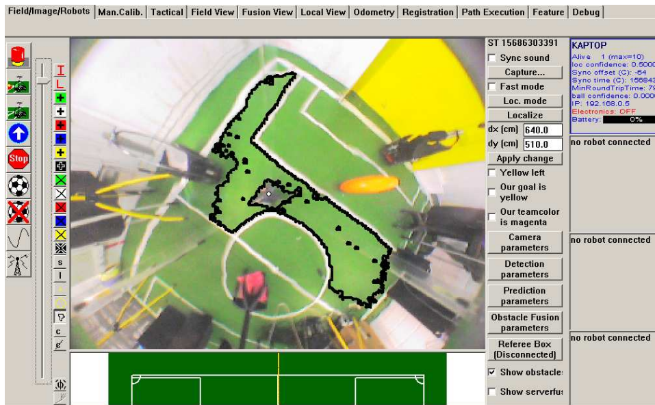
Figure 1.4: The manual color calibration tool of the FU-Fighters system. The operator clicks a point in the image where a color growing should be started with a manually chosen threshold. The pixels are compared to the starting point and added to the region until they exceed the given threshold. The operator then adds the region to the corresponding color class or chooses another region.
