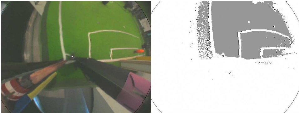
Figure 4.1: The classification (on the right) was obtained after a few second with no previous classification. Here the ball and the goals are too far away to be calibrated so only the field can be calibrated. The color code is: white = unclassified, gray = field.
