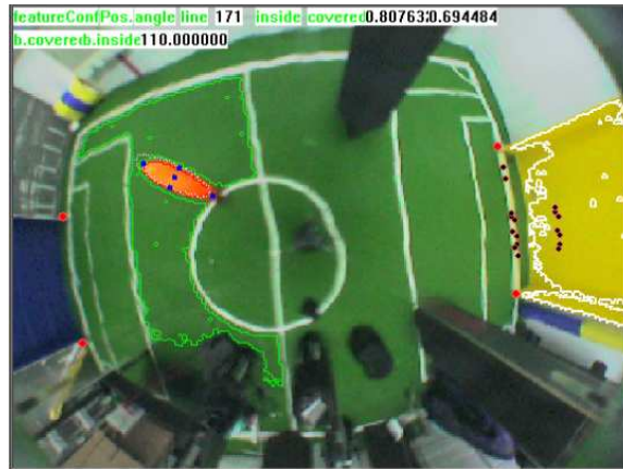
Figure 3.3: Regions grown successfully for an expected ball region, one of the expected field regions, and an expected goal region. The grown goal region is enclosed by a white curved line, the ball's by a red curved line and the field's by a green curved line.
