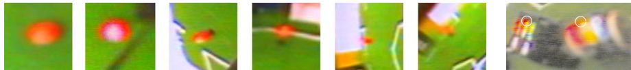
Fig. 5. The ball's appearance varies in color and shape and is similar to robot markers.
