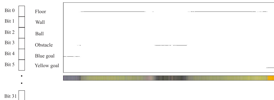
Fig. 2. Color classification of the pixels belonging to the line in Figure 1(c).
